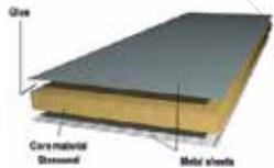
Sandwich panels for building applications are large prefabricated building products.
